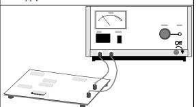
Turning off power to the circuit under test would only prevent damage that might occur if you accidentally short two lines together while connecting probes. You can leave the HP 54645A/D powered on because no voltage appears at the probes.
