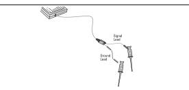
**6** Connect the ground lead on each set of channels, using a probe grabber. The ground lead improves signal fidelity to the instrument, ensuring accurate measurements.
