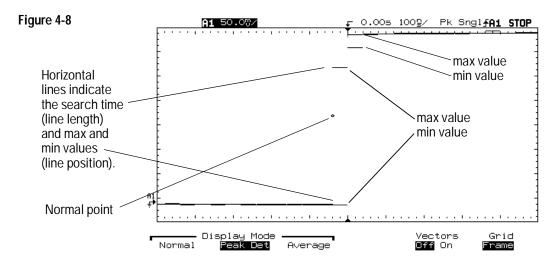
**Resolution Limit in Peak Detect with Vectors Off**
