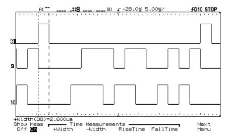
Positive Width Measurement on HP 54645D Digital Channels
