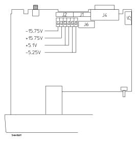
**Low Voltage Power Supply Voltage Test Points**
