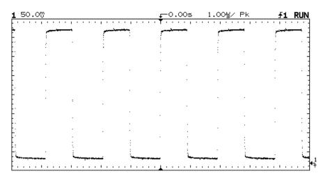
Simple Square Wave in Peak Detect Mode on HP 54600
