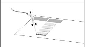
5 For high-speed signals, connect a ground lead to the probe lead, connect a grabber to the ground lead, and attach the grabber to ground in the circuit under test.
