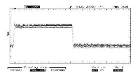
**Asynchronous Noise in Pulse**
