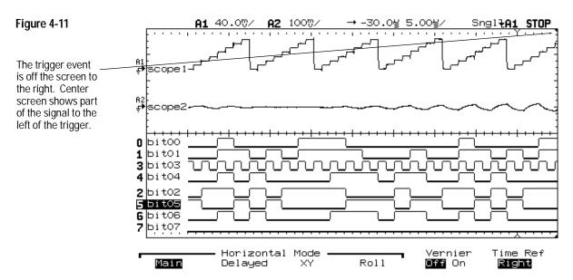
If we set the time reference to center, then pan the display back to set the delay to 0  $\mu$ s, the trigger point is displayed at center screen, and the result resembles:
