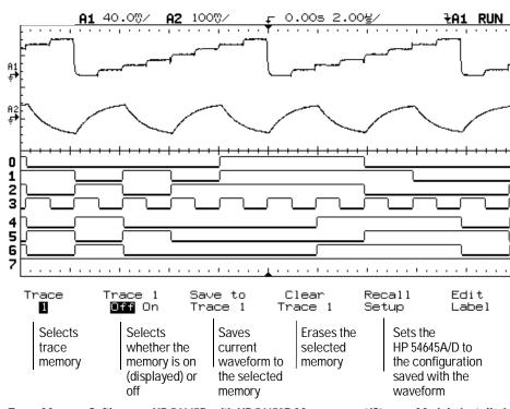
Trace Memory Softkeys on HP 54645D with HP 54659B Measurement/Storage Module Installed
