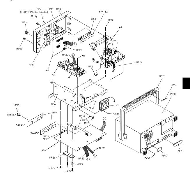
Exploded View of HP 54645A/D Oscilloscope
