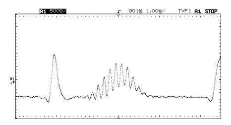
Modulated 12.5T Pulse on the FCC Composite Test Signal
