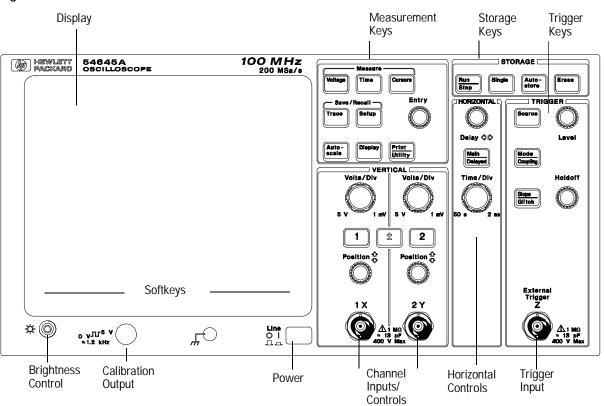
HP 54645A Oscilloscope Front Panel
