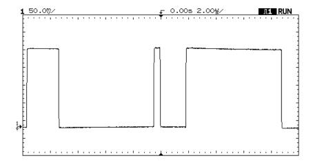
HP 54645A Triggered on Glitch on Channel 1
