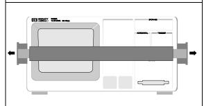
**2** Without releasing the pivots, swivel the handle to the desired position. Then release the pivots.
