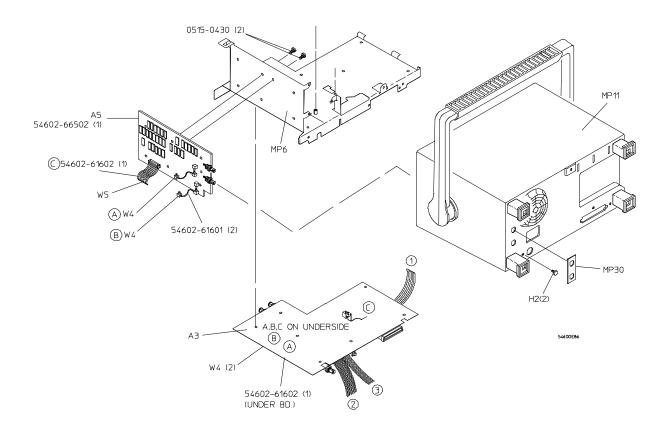
Exploded View of Option 005 and Related Oscilloscope Parts
