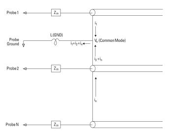
Common Mode Input Voltage Model
