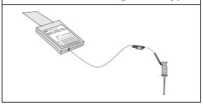
**4** Connect the grabber to a node in the circuit you want to test.
