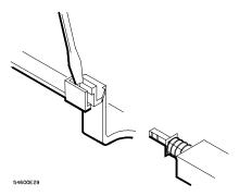
**Unhooking the Power Switch Shaft**
