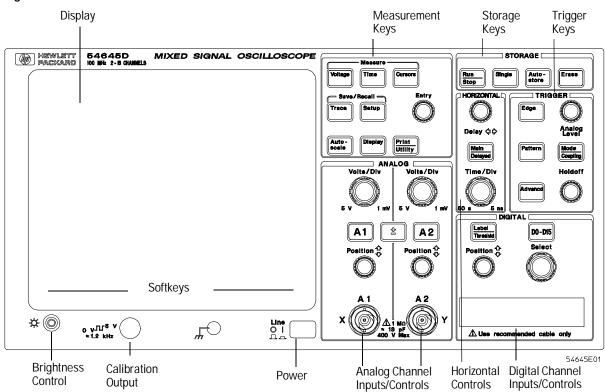
HP 54645D Mixed-Signal Oscilloscope Front Panel
