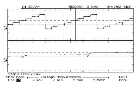
**Isolating Area for Vtop Voltage Measurement**
