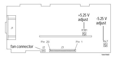
Low Voltage Power Supply Adjustment Locations (top side of oscilloscope)
