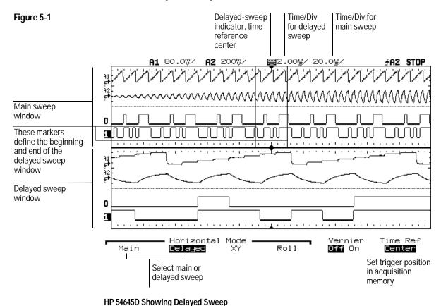
The screen divides in half. The top half displays the main sweep, and the bottom half displays an expanded portion of the main sweep. This expanded portion of the main sweep is called the delayed sweep. The top half also has two solid vertical lines called markers. These markers show what portion of the main sweep is expanded in the lower half. The size and position of the delayed sweep window are controlled by the Time/Div and Delay knobs.
