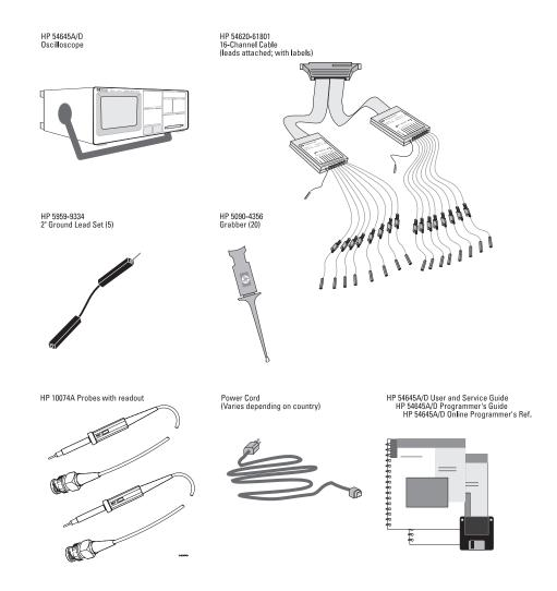
Items Supplied with the HP 54645A/D Oscilloscopes
