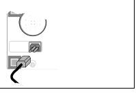
The HP 54645A/D power supply automatically adjusts for input line voltages in the range 100 to 240 VAC. Therefore, you do not need to adjust the input line voltage setting. The line cord provided is matched by HP to the country of origin. Ensure that you have the correct line cord. See table 1-1.
