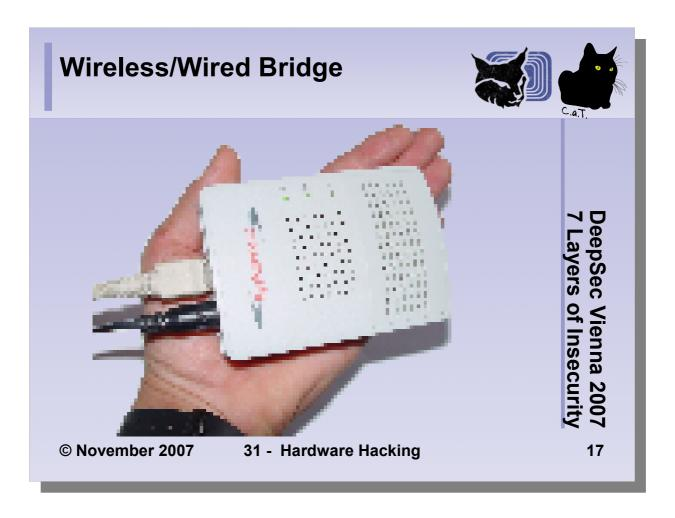
The device shown in the picture is a miniature access point. It can act as a bridge between the connected Ethernet and the wireless network. This mode can be activated with a single switch located on the side of the device.
