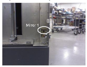
A. Stand on the right hand side of the machine looking at the side of the machine. If you look at the lower right hand corner of that side of the machine you will see a rectangular cut out in the frame of the machine. If you look through that cut out and you will see a thumb screw with three allen head screws in the form of a triangle around the thumb screw. Those are the adjustment screws for mirror one (Picture Above).
