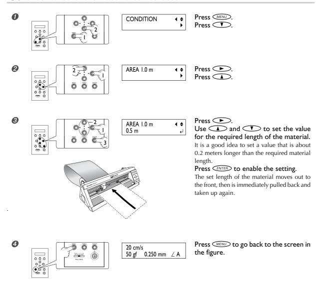
If the material comes loose from the pinch rollers, press the [PAUSE] key to stop operation. Then reload the material, starting over from the beginning.
