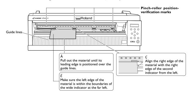
**3** Move the pinch rollers so that they are positioned at the edges of the material and also inside the areas of the pinch-roller position-verification marks.
