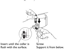
Support the screw from below and insert the blade holder.
