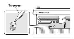
Press to feed the material toward the front, then use the included tweezers to peel off the cut shapes and check the cutting quality.
