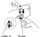
Support the screw from below and insert the blade holder.
