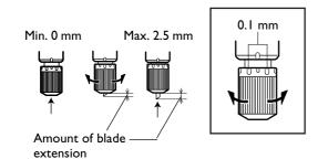
When you want to perform accurate and fine adjustment of the cutting-in amount, such as when cutting media with thin carrier paper, you can obtain good results by adjusting the tip of the blade.
