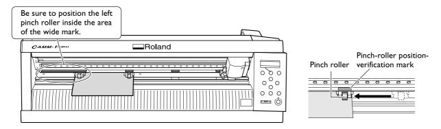
Be careful to position the pinch rollers so that they are not too close to the edges of the material and do not extend beyond the edges of the material.
